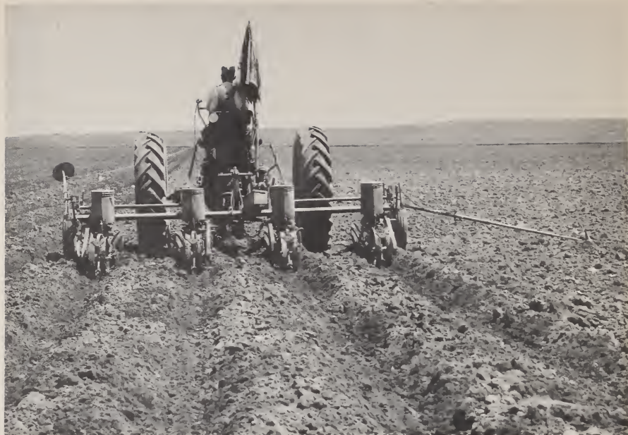
FIGURE 2.—Planting grain sorghum with a loose-ground, furrow-opener planter. This machine has many of the advantages of both surface planting and listing.
